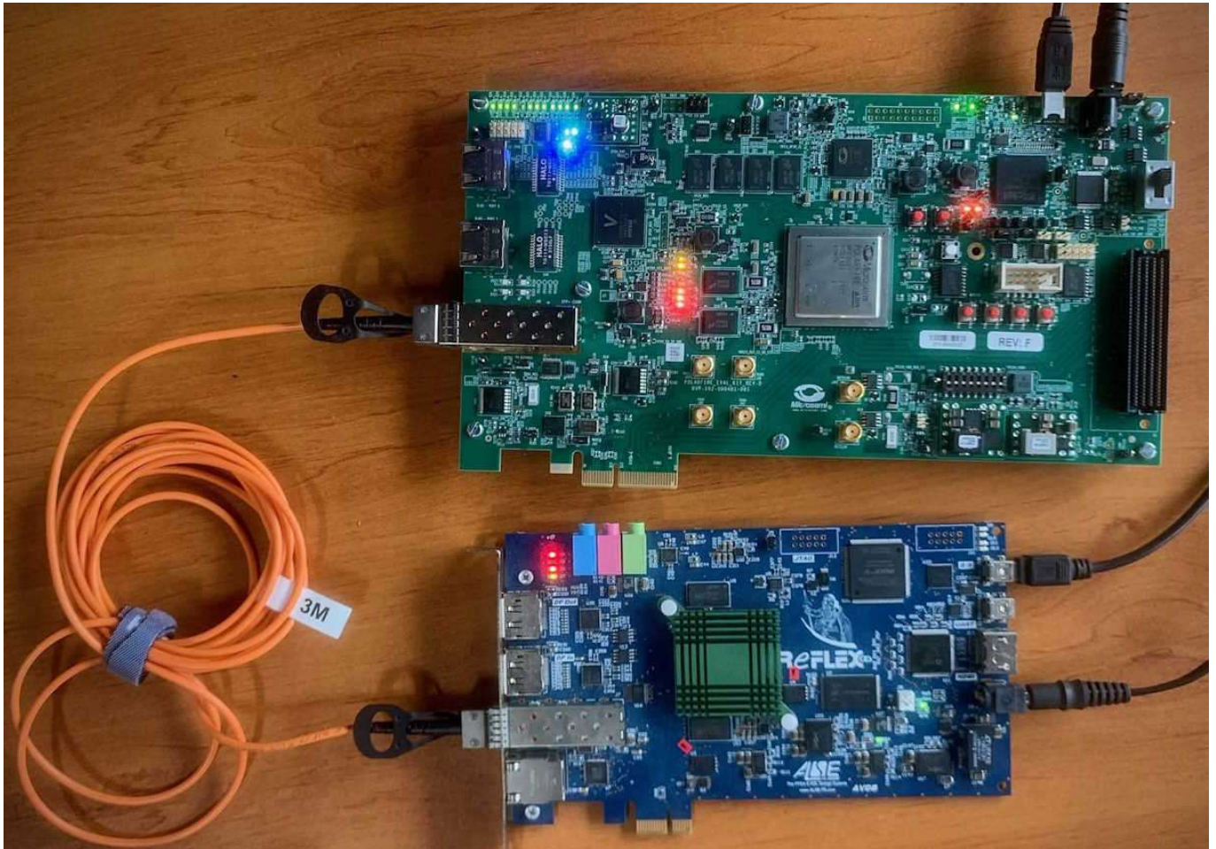
Figure 3 : x1 lane hardware test bench overview
